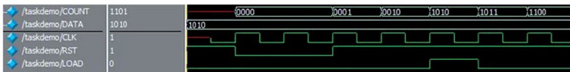
■ FIGURE 6.3 Simulation of parallel call to task TOGGLE
