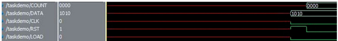
■ FIGURE 6.8 Simulation of serial call to task TOGGLE with local variable CLK
